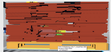
Sample view of a staple after commissioning with optimised sorting and positioning.
